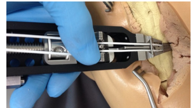
H. Push free cable ends into cleat.
